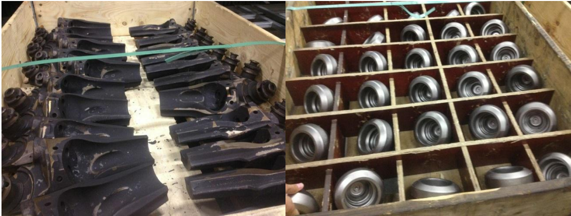
Picture 4, To the left: legs before blaster. To the right: rolls after blaster.
